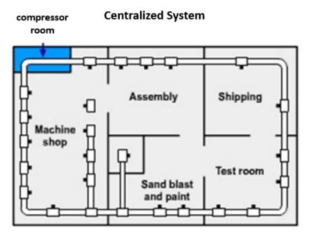
Figure 4.15 Centralized system layout
