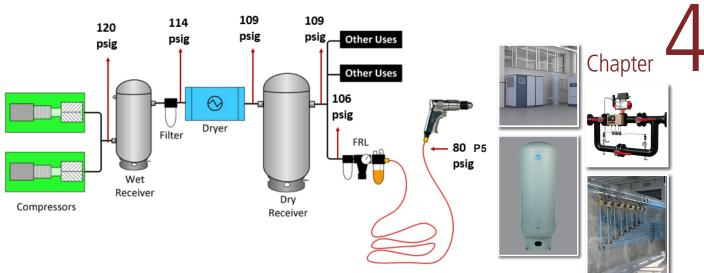
Figure 4.6 Start P2 compressor selection with an analysis of P5 critical pressure
