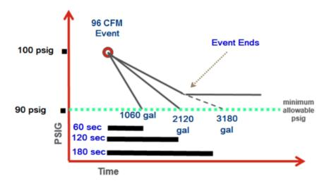
Figure 4.22 Effect of control storage on rate of change
