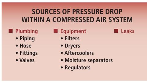
Figure 4.4 Common sources of pressure drop
