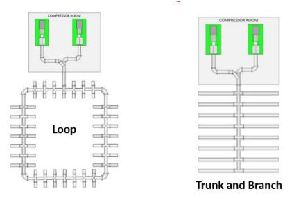
Figure 4.17 Two basic distribution piping layouts
